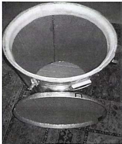
Faraday Cage with cardboard lining in can and lid
